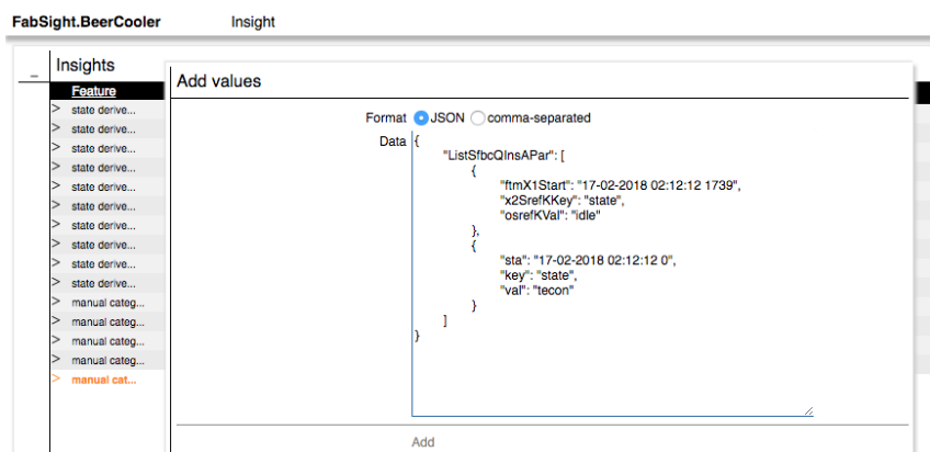
Figure 5: JSON entry of insight values, template for API-based procedure
